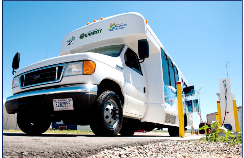
National Renewable Energy Laboratory. A Ford hydrogen-powered internal combustion engine (H2ICE) bus at the National Wind Technology Center.
